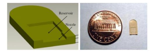
The self-propelled microboat takes advantage of the surface tension difference in the front and back of the boat when isopropul alcohol leaks from the back reservoir. The microboat can reach speeds of 30 cm per second. Credit: Cheng Luo, et al.
