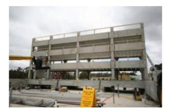
Engineers at UC San Diego's Englekirk Center are testing the seismic response of precast concrete floor systems that are used in parking garages, college dormitories, hotels, stadiums, prisons and increasingly in office buildings.
