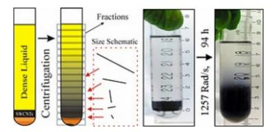
In a schematic of NIST's length separation technique for carbon nanotubes (l.), the nanotubes start at the bottom of a dense fluid. When spun in a centrifuge, the nanotubes begin to migrate through the fluid driven by their buoyancy, but the longer ones move faster, spreading them out by length. Photos (r.) shows a typical sample at the start and after 94 hours of spinning at 1257 radians per second (roughly 12,000 RPM). Credit: NIST
