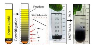
In a schematic of NIST's length separation technique for carbon nanotubes (l.), the nanotubes start at the bottom of a dense fluid. When spun in a centrifuge, the nanotubes begin to migrate through the fluid driven by their buoyancy, but the longer ones move faster, spreading them out by length. Photos (r.) shows a typical sample at the start and after 94 hours of spinning at 1257 radians per second (roughly 12,000 RPM). Credit: NIST
