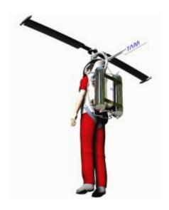
Technologia Aeroespacial Mexicana (TAM) has designed a strap-on helicopter. Tiny rockets on the tips of the propellers eliminate the need for a tail rotor, making it possible for the device to be worn on a human body. Credit: TAM.
