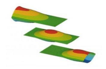
The novel micro-pump works in a similar way to the human esophagus: The liquid is ingested from the left (above), propelled forward by contractions of the pump (center) and released on the right (below). Credit: Fraunhofer IWM
