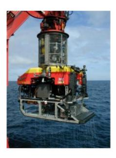
The ISIS robot which will be used by scientists to collect rock samples from volcanoes on the Mid-Atlantic Ridge two miles (3km) below the surface of the sea. Photograph courtesy of the Natural Environment Research Council
