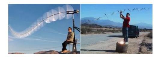
(Left) Doug Selsam with a prototype 25-rotor turbine that can generate 3,000 watts, while the other end is held up by a balloon. Credit: Popular Science. (Right) Selsam holds a model with 14-inch rotors that can power the 50-watt headlight at his feet. Credit: SpeakerFactory.net.
