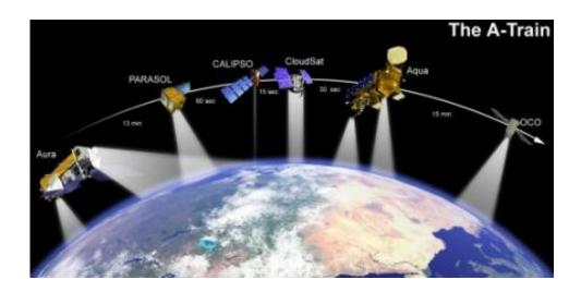
This artist's concept shows how the satellites composing the A-Train fly in formation to make near-simultaneous observations of Earth. Credit: NASA
