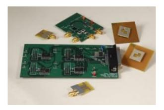
Components of the testbed Georgia Tech's Gregory Durgin developed to simultaneously measure hundreds of radio frequency identification RFID tags and rapidly test new RFID tag prototypes. Georgia Tech Photo: Gary Meek
