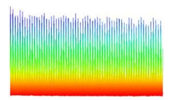
Experimental data from a NIST "gap-toothed" frequency comb that are false colored to indicate the range from low power (red) to high power (blue). The comb is specially designed for astronomy. Each "tooth" is a precisely known frequency, and the teeth are widely separated (by 20 gigahertz) in comparison to a standard comb. Credit: M. Kirchner & S. Diddams/NIST
