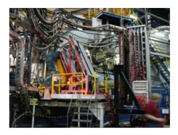
Correlated protons and neutrons were measured in the BigBite large acceptance spectrometer (blue/gold magnet with detector package) and a neutron detector (tall assembly at right).
