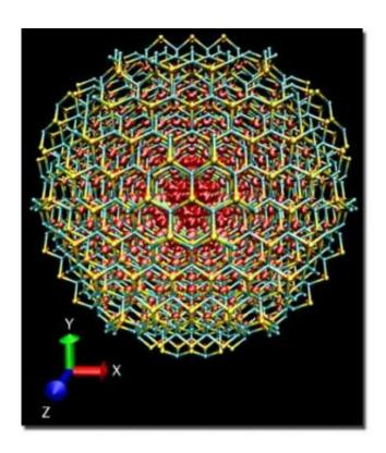
Fluorescence from CdSe quantum dot solids in environments varying from stable to high unstable show that small deviations from uniform stress distribution greatly affect the electronic properties. The blue represents cadmium, the yellow represents selenium and the red represents a cloud of electrons in their excited state. Image by Sebastien Hamel/LLNL
