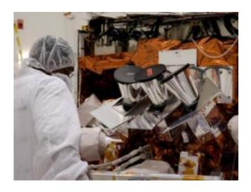
At the Astrotech payload processing facility near Kennedy Space Center in Florida, a worker looks over the star tracker sun shades just installed on the GLAST spacecraft. Credit: NASA/Kim Shiflett
