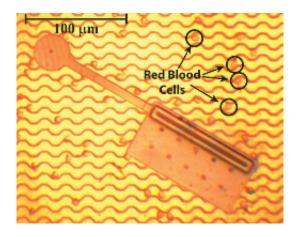
A photograph of a typical nanosoccer robot compared in size to red blood cells. About 200 of these robots could stretch in a line across the top of a plain M&M candy. Credit: Craig McGray
