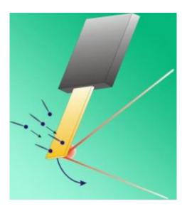
NIST researchers measured the surface stress of a monolayer film on gold by measuring the changing curvature of a gold-coated glass cantilever as molecules of mercaptobenzoic acid were deposited on the gold. The change in curvature was detected by the shifting reflection of a laser beam impinging onto the back side of the glass. Credit: NIST
