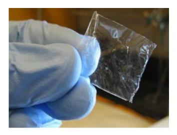
The new, thin material developed by MIT engineers for use in methanol fuel cells. Photo courtesy / Avni Argun and Nathan Ashcraft, MIT
