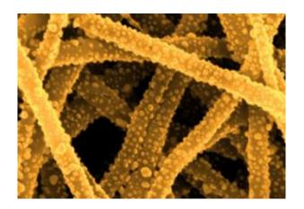
Nylon nanofibers coated with metal nanoparticles. These functional nanofibers have potential applications as active air filtration media as well as flexible antibacterial surfaces such as wipes, carpets and upholstery.
