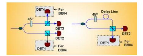
A highly simplified schematic of a recipient's detectors in a quantum cryptography setup. Conventional cryptography setups (left) require at least two detectors, and the most common setup, known as BB84, requires four. By adding an optical component that delays the travel of photons to the detector, the number of required detectors is cut in half. Credit: NIST
