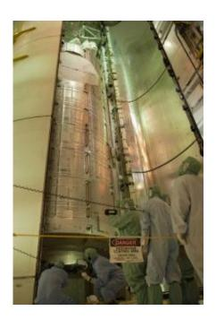
Workers in the payload changeout room on Launch Pad 39A at NASA's Kennedy Space Center check the placement of space shuttle Discovery's payload bay doors as they close around the Japanese Experiment Module - Pressurized Module. Photo credit: NASA/Kim Shiflett
