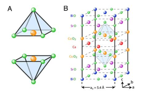
Cuprate crystals consist of layers of copper oxide interleaved with layers of other atoms. Copper and oxygen atoms usually form a pyramid with the oxygen atom at the apex located in an adjacent layer. Cornell research now shows that other atoms pushing that oxygen out of position creates superconductivity.
