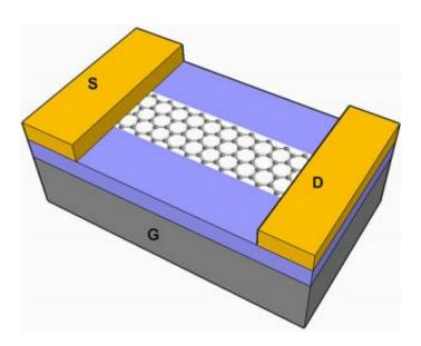
A schematic of graphene nanoribbon field-effect transistor with palladium contacts (S,D) on a 10 nm thick insulating silicon dioxide surface (purple). Beneath the Si02 layer is a highly conductive silicon layer (G). Credit: Stanford University
