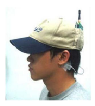
The brain-computer interface consists of a baseball with six electrodes (one under the left ear) that detect the wearer's EEG signals. In the current prototype, the system can detect brain activity that corresponds with a person's drowsiness level. Credit: Chin-Teng Lin, et al. ©2008 IEEE.
