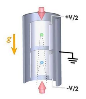
The neutrality test experimental setup, showing the atoms&acute trajectories.
