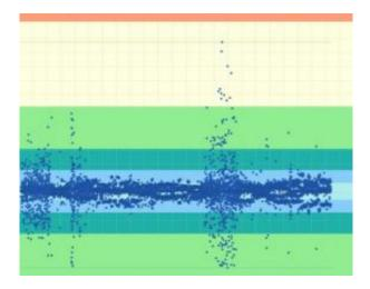
The points on this graph from the EtherNet/IP Performance Test Tool represent data packets. Those points pictured away from the centerline reflect timing errors in the network communications of the device being analyzed. Credit: NIST
