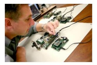
Kevin Carr, an undergraduate in electrical and computer engineering, adjusts one of the transmitter modules that is used to wirelessly link five units being tested in a self-healing computer system. The unit to the left of the transmitter is a Field Programmable Gate Array. Other transmitters and FPGAs can be seen in the background. (Photo by Matt Brailey)
