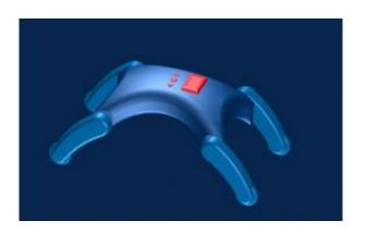
This artist's drawing shows the ground-based robot that Hariri is developing for the project at Biosphere 2. The robot will have four wheeled "leg-like" structures that will help it adapt to terrain. (Illustration: M. Anthony Lewis)
