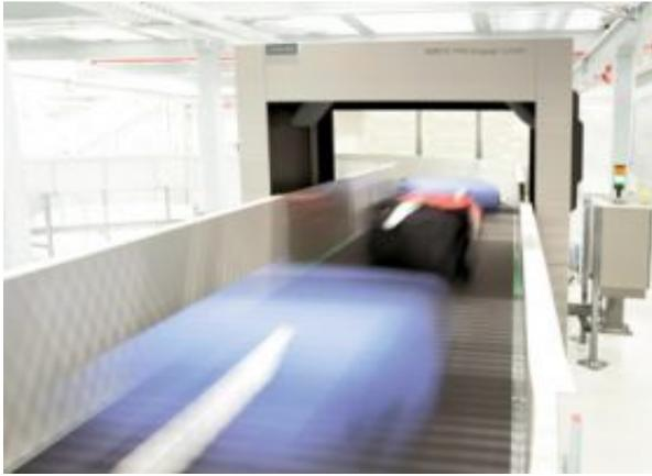
Transporting passenger baggage between the world's airports is expected to become far more reliable in the future — with RFID technology. Siemens has developed a system that relies on a radio chip to replace the bar code attached to a suitcase. The new technology will substantially reduce scanning errors and resulting sorting and delivery errors.
