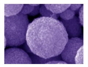
A close-up of a single ball, taken with a scanning electron microscope. The 300-nanometer sphere is large enough to scatter light. But its insides are made of tiny grains just 15 nanometers across. Credit: University of Washington
