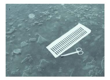
An equal sized hole in the ice, this time with a polymer raft placed in it. Fifteen minutes later, the ice is thick enough to support the scissors&acute weight.
