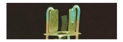
The thumbnail-sized patch of "window screen" suspended between the electrodes is the paddle that stirred the CVX-2 xenon sample.
