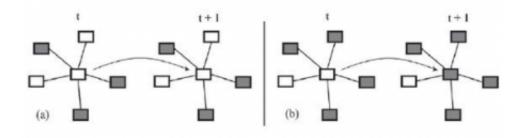
The model updates the state of a node (individual) depending on the fraction of the states of its neighbors. In this case, that fraction ("laggard parameter") is 80%. In (a), the central node keeps its original state. In (b), the central node is updated since 80% of its neighbors are in the opposite state. Credit: P. Klimek, et al.
