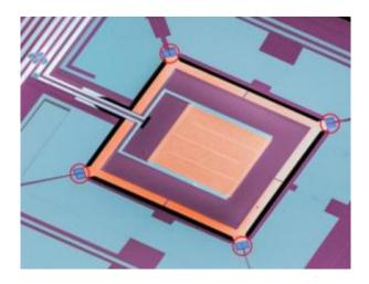
Colorized micrograph of a NIST chip combining four microrefrigerators (circled in red) with a superconducting sensor (large orange square in the middle). The self-cooling chip could be used for applications ranging from detailed X-ray analysis of semiconductors to detection of microwave signals in deep space. Credit: Credit: N. Miller, K. Talbott NIST
