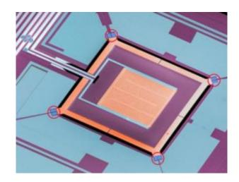
Colorized micrograph of a NIST chip combining four microrefrigerators (circled in red) with a superconducting sensor (large orange square in the middle). The self-cooling chip could be used for applications ranging from detailed X-ray analysis of semiconductors to detection of microwave signals in deep space. Credit: N. Miller, K. Talbott NIST
