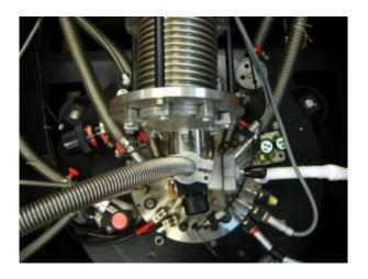
To perform the experiment, the researchers used a dilution refrigerator, a device in which the temperature can be lowered to several millikelvin, just above absolute zero. The thin superinsulating films are then placed in the camera of the dilution fridge. Credit: ANL
