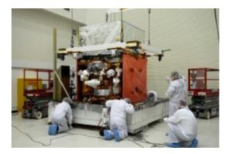
At the Astrotech payload processing facility, General Dynamics technicians check GLAST before the installation of the solar arrays, as an overhead crane is lowered over it. Credit: NASA/KSC
