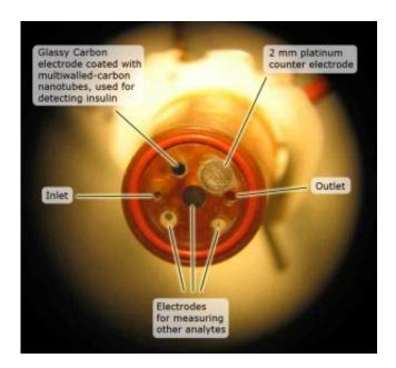
Close-up of the new sensor that can measure the concentration of insulin produced by Islets of Langerhans cells at the same time as it measures other compounds that allow the researchers to assess cells' healthj. Credit: Cliffel Laboratory
