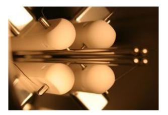
The orientation of the molecules decides whether they will reach the end of this open tube. The electric field between the four metal rods changes constantly so that only conformers with the correct mass-to-dipole-moment ratio can pass through the open tube. Image: Fritz Haber Institute of the Max Planck Society
