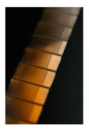
An experimental near-field plate is a patterned grating like surface that can focus electromagnetic waves to subwavelength resolutions. Photo by Cyan James
