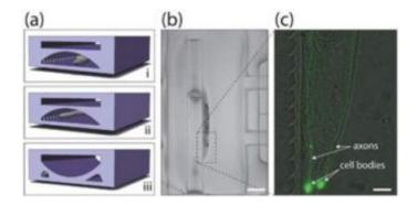
Figure illustrates "lab on a chip" technique developed by MIT researchers to allow immobilization and imaging of a live C. elegans worm: (a-i) worm moves freely in chip's microfluidic channel; (a-ii) partial immobilization of worm; (a-iii) full immobilization; (b) low magnification image of worm immobilized in the device; (c) close-up of immobilized worm showing animal's neurons (fluorescent). Image courtesy / Mehmet Fatih Yanik
