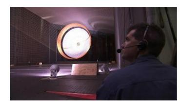
This image shows a perfectly functioning parachute with the canopy fully open at the opposite end of the wind tunnel after being fired from the cannon. Image credit: NASA
