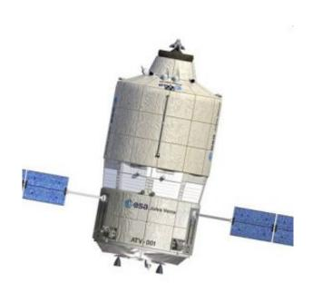
The Automated Transfer Vehicle (ATV) is the first fully automatic re-supply spacecraft of its kind. ESA's Jules Verne ATV is the first European space supplier for the ISS. It was launched 9 March 2008 from Europe's spaceport in Kourou, French Guiana. Credits: ESA - D.Ducros
