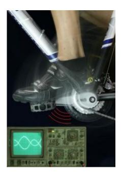
Adaptronic elements cast in the pedal crank report inappropriate biomechanical stress during cycling. Credit: Fraunhofer IFAM
