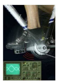
Adaptronic elements cast in the pedal crank report inappropriate biomechanical stress during cycling. Credit: Fraunhofer IFAM
