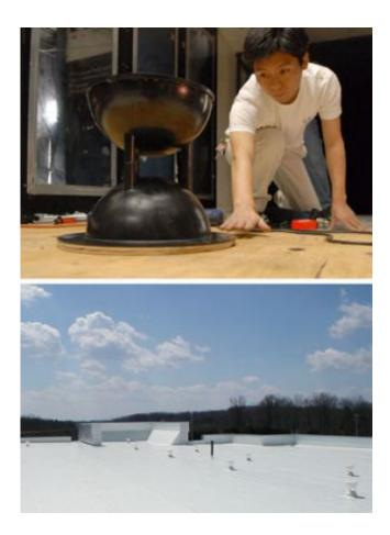
(top) Engineering science and mechanics doctoral student Yihong Yang installs the V2T prototype roof vent in the Virginia Tech stability wind tunnel. Photo courtesy of Michael Miller, Virginia Tech Intellectual Properties. (bottom) One of the buildings on which the V2T roof system is in use is KnowledgeWorks in the Virginia Tech Corporate Research Center. Photo courtesy of Pat Johnson, Acrylife.
