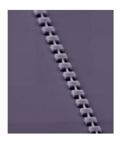
A section of the coupled-resonator slow-wave structure in silicon fabricated using electron-beam lithography. The full structure consists of one hundred coupled cuboidal resonators connected sequentially by a thin photonic-wire waveguide. Credit: UC San Diego
