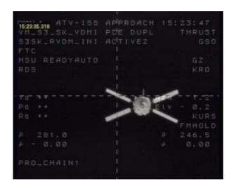
This image captured from the ESA Docking Video System used by astronauts and mission controllers to monitor ATV's approach to the ISS during Demonstration Day 2, 31 March 2008. Credits: ESA
