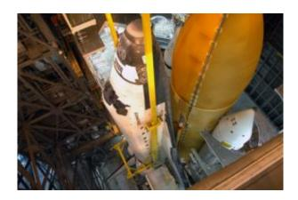
Space shuttle Discovery is lowered into position beside its external tank and solid rocket boosters inside the Vehicle Assembly Building at NASA's Kennedy Space Center in Florida. Photo credit: NASA/Jim Grossman
