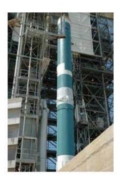
On Pad 17-B, the mobile service tower (left) approaches the Delta II rocket (right). The solid rocket boosters in the tower will be mated with the rocket. Credit: NASA/Jim Grossmann
