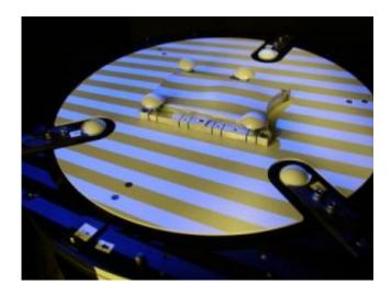
A mathematical method analyzes the distortion of the stripes, enabling errors in the manufacturing process to be rapidly identified. Credit: Fraunhofer IOF
