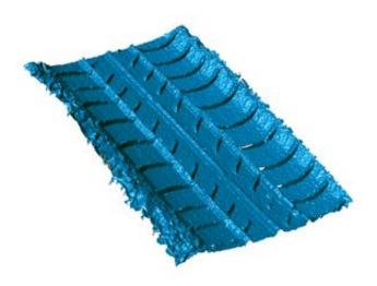
A 3-D sensor enables the tracks left by car tires (right) to be quickly and easily imaged. © Fraunhofer IOF
