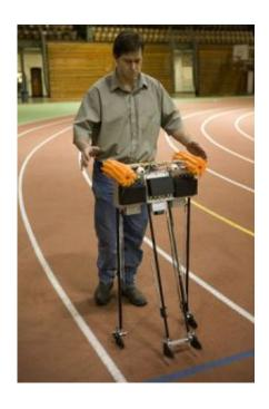
Jason Cortell, manager of the Biorobotics and Locomotion Lab, follows the Cornell Ranger, on a test walk. The robot's body hides complex computer controls that sense the position of the legs to decide when to swing them forward and how to adjust the pivoting feet. Photo: Jason Koski
