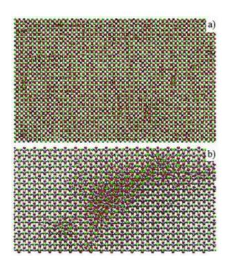
In yttria-stabilized zirconia (top), the defects produced by radiation are few and far between, having less impact on the properties of the material. In zircon (bottom), the defects are clustered, which could compromise the material's integrity. Credit: PNNL
